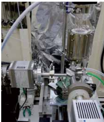
図1 Tender X-ray in-situ XAFS(蛍光) cell
