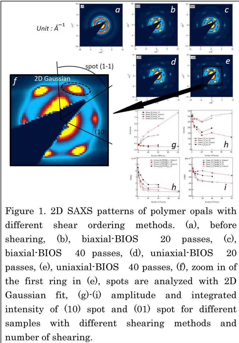
The measurements are performed using the photon energy of 8.2 keV and a Rigaku high resolution detector. The radius of the beam stop is just at the edge of an acceptable level for imaging the reciprocal space lattices, which gives us as much information as we want but at the same time generated some distortions over the diffraction patterns.
