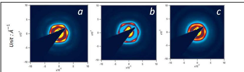
Figure 2. 2D SAXS patterns of binary polymer opal films ordered with uniaxial 20 passes. (a),  $R_L:R_s = 1.2$ , (b),  $R_M:R_s = 1.2$ , (c),  $R_L:R_s = 1.4$
