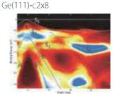
Energy dependence of ARPES specta measured with synchrotron radiation reveals the origins of spectral features. Features S1-S3 are located in the same energy for different excitation energy excitation, and attributed to surface states Additional features observed only for ARPES spectrum of Ge-Bi $\sqrt{3}$  were assigned as the surface states derived from Bi.
