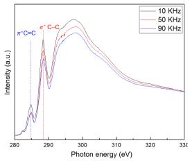
Figure 2 NEXAFS spectra of NDC films deposited at negative bias frequency of 10 KHz (black), 50 KHz (red), and 90 KHz (blue).
