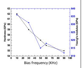
Figure 1 Dependence of hardness and Young's modulus on negative bias frequency.
