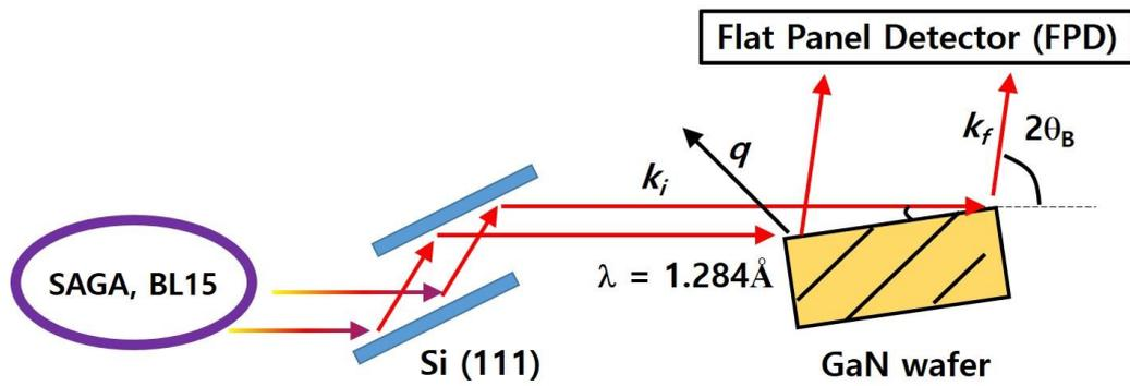
Figure 1. Schematic view of the experimental configuration. X-rays of  $1.284\text{\AA}$  were selected by Si (111) double crystal monochromator. GaN wafers were put in the rotation center. A flat panel detector was placed at Bragg angles, and diffraction images were recorded at various incident angles.
