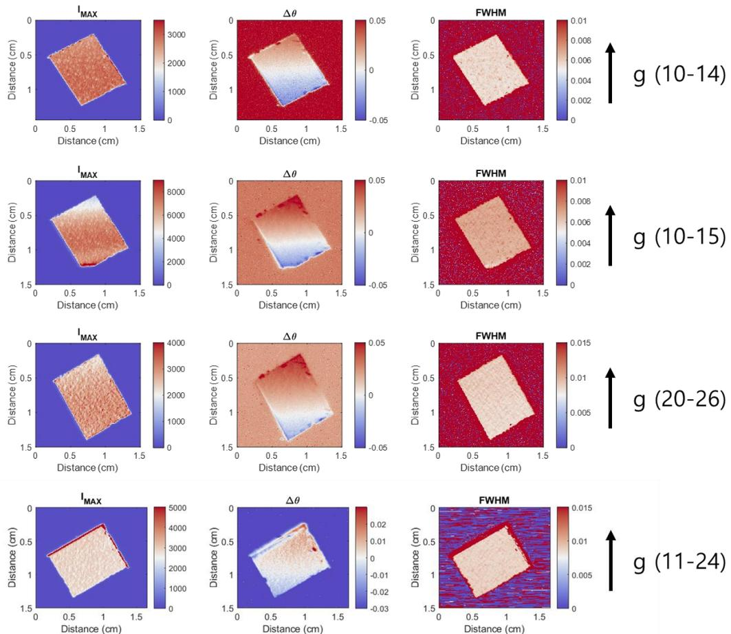
Figure 2. Merged x-ray diffraction topography images of c-plane GaN under different g-vector. The maximum intensity, peak position, and FWHM of each pixel are strongly dependent on the g-vector. The unit in peak position image is degree.
