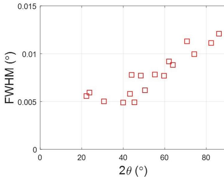
Figure 1. X-ray rocking curve width as a function of  $2\theta$ . The FWHMs were increased as a function of  $2\theta$ .
