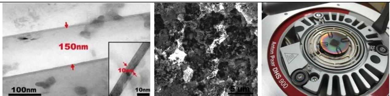
**Figure 1.** The microstructures of the composites (Left) Al-Al<sub>2</sub>O<sub>3</sub>-GrO (the inset shows a Al<sub>2</sub>O<sub>3</sub>-GrO-Al<sub>2</sub>O<sub>3</sub> sandwiched layer) and (Middle) Al-GrO. (Right) The furnace used for heating up in in-situ experiments
