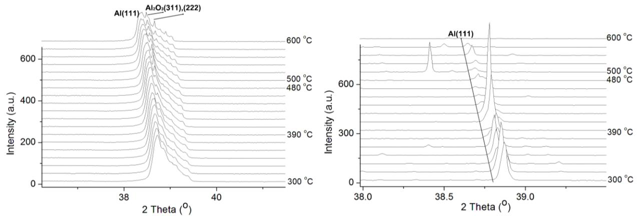
**Figure 3.** The characterized  $2\theta$  range reflecting the phases changes in the composites of (Left) Al- $\text{Al}_2\text{O}_3$ -GrO and (Right) Al-GrO.
