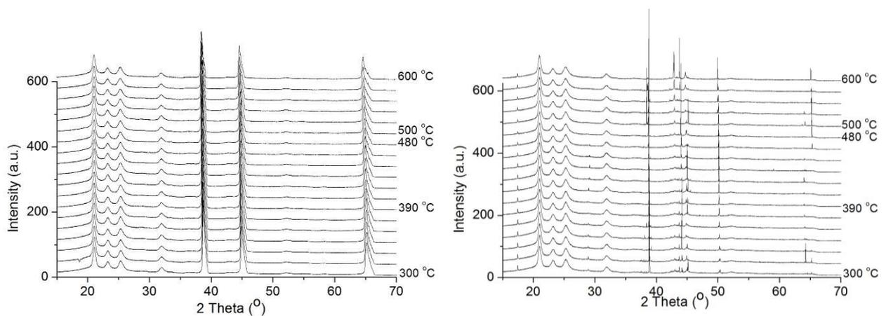
**Figure 2.** The spectra collected from the in-situ diffraction experiments for the composites of (Left) Al-Al<sub>2</sub>O<sub>3</sub>-GrO and (Right) Al-GrO.
