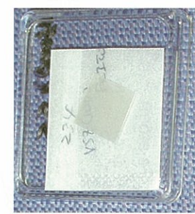
Fe@ITO thin film on YSZ substrate deposited by PLD.
