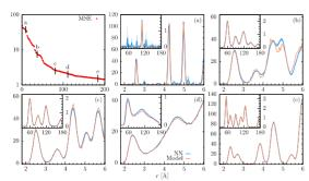
Performance of the trained NN on the test dataset. On the top left, the Mean Square Error (MSE) of the worst 200 cases are shown in descending order. Predicted RDF and BAD (insets) from selected configurations are shown in blue and the shadowed area represent standard deviation of the predictions. Orange lines are the same quantities calculated from the models, which are: (a) dia, (b) hcp, (c) fcc, (d) liquid and (e) bcc.
